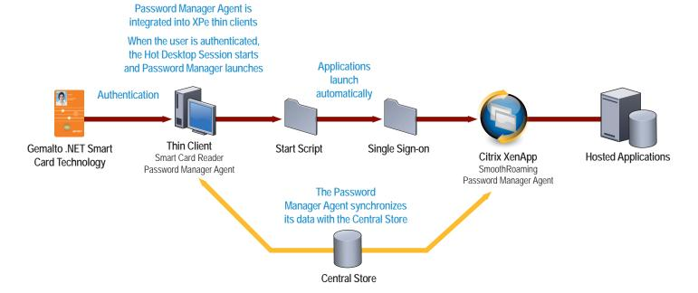
.NET-powered smart card runs a small footprint version of the .NET Framework to provide customizable two-factor authentication. For still greater security—and convenience—Gemalto eliminates the need to keep track of multiple identification cards and passwords. For example, the same .NET smart card a clinician uses for network access via a thin client can also be used for physical access into the hospital. It can even be personalized with a picture and other imprinting to prevent forgery.
